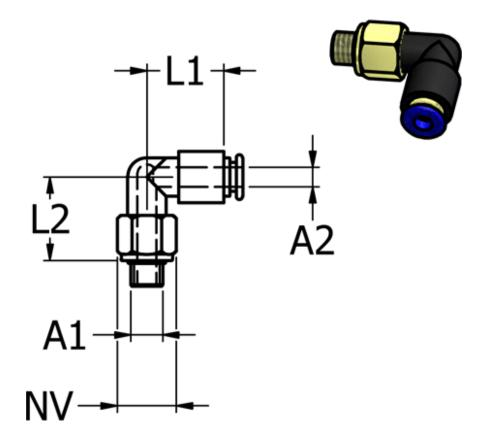
Ext. hose diameter A2 = 4 mm L1 = 14 L2 = 17.6 NV = 10 Thread A! = M6
